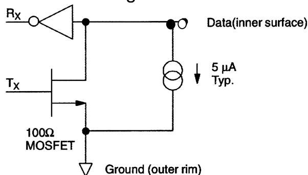
**BUS MASTER CIRCUIT Figure 3****A) Open Drain**
